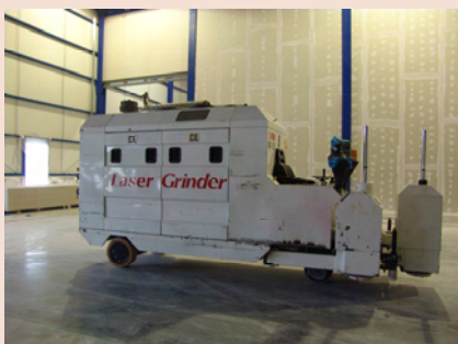
The laser grinder ready to work without racking being present
