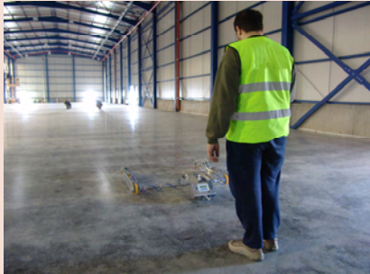
Face consultants survey the floor according to DIN 15185 before the racking installation
