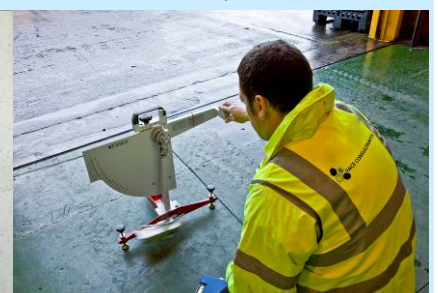
Slip /Skid Resistance Testing
