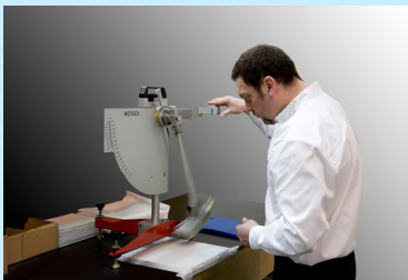
Duane with Slip/Skid Resistance Tester in a laboratory environment.
